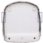
16) With a fine razor saw, cut off the molded on buffer beams level with the bottom of the ends. Use the underside of the end as a fence to guide the saw blade and finish off with a flat file to remove any burrs.
